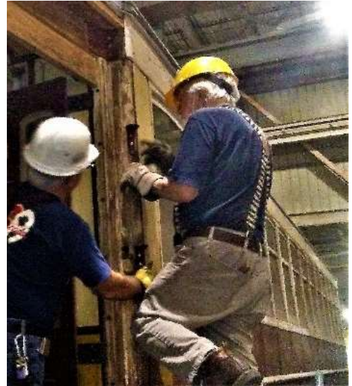
Tony is joined by Jim Houston in replacing half-round moldings to side panels. (Photo by Marc Lipkin)
