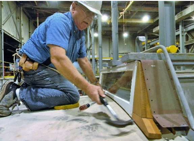
Now that canvas is in place, the assembly of the roof end route sign box can be addressed. Here, Jim demonstrates his chops as "car knocker par excellence."
