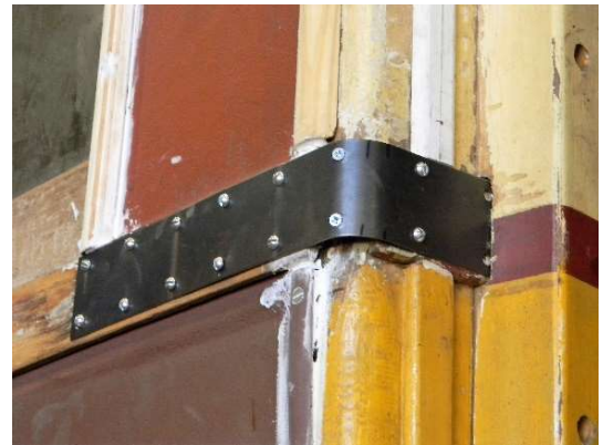
No, NOT the battleship NEW JERSEY, just one of four corner plates re-manufactured by our friends at Kinkisharyo LLC from a rusted out original and installed by Tony.
