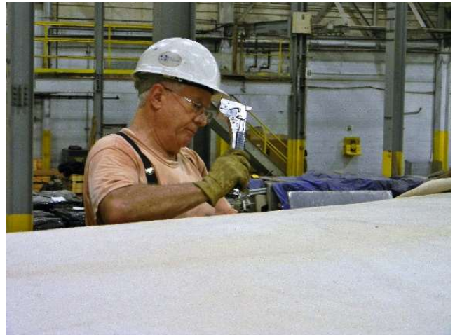
Jim uses staples to temporarily hold the canvas in place during the working.
