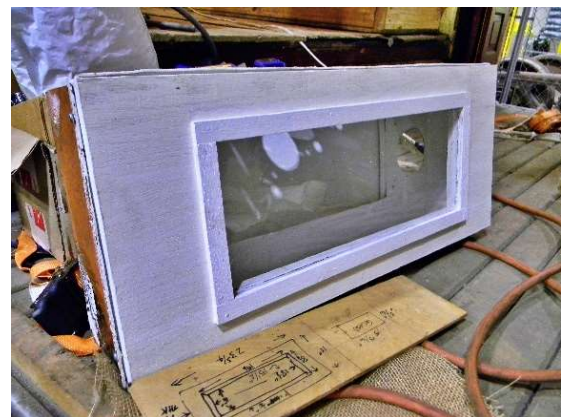
A new sign box cover was made up by Jim Houston, replicating the one at the "A" end, built by Tony at P-Burg years ago.
