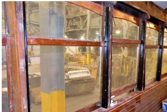
Thanks to RM Auto Restorations of Windsor, Ontario and the good offices of friend and Charter Member Dave Phraner, three pairs of complex window channels were custom manufactured for us at an affordable price. Fortunately for us, RM had just completed a "Williamsburg" level restoration on former RL&RR #351, a car identical to 2651 (See Trolley Lines #31). They had wisely, and for us fortunately, retained the dies they had created for their project!
