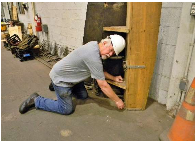
New contributing member and avid volunteer Jeff Wewers is seen here disassembling the temporary steps fitted at P-Burg to facilitate easier access while the car is blocked high on its trucks for easier access to underfloor equipment.
