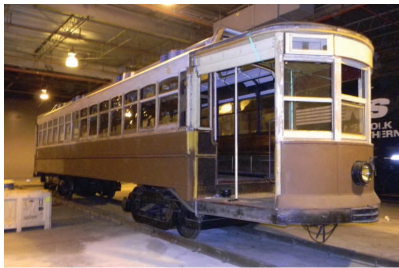
Figure 35: In a short time 2651 was once again enjoying a solid roof overhead. Trolley poles and steps were transported on board, life guards separately in the case at left. Photo: Tony Hall DSCN3228
