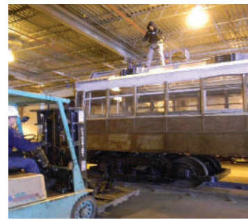
Figure 81: KS staffer Esteban is already on the roof, waiting for the palletized pole base to be raised. Photo: DSCN3277
