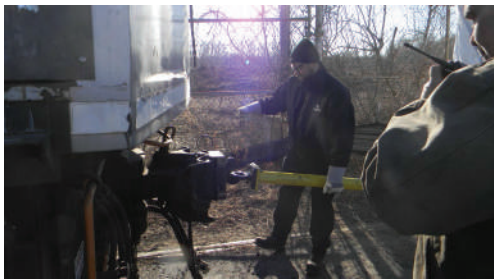
Figure 68: Using a unique drawbar of their own design, KS crew couples #1 to ERDX 4139 (ex-NJ Transit) Photo: DSCN3124
