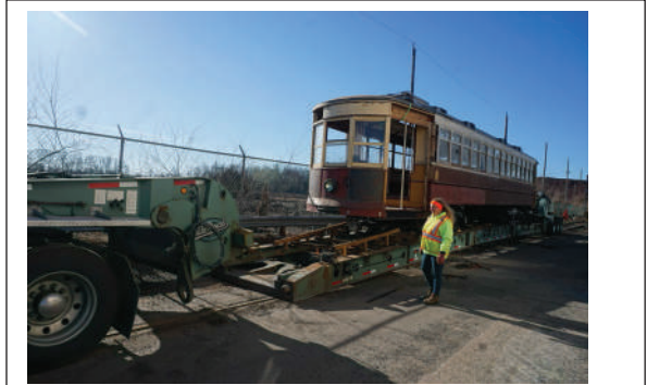
Figure 33: The Tractor Cab has been uncoupled, the unloading ramp will be deployed. And, 2651 will once again take to permanent rails. Photo: Bob Hooper DSC0485
