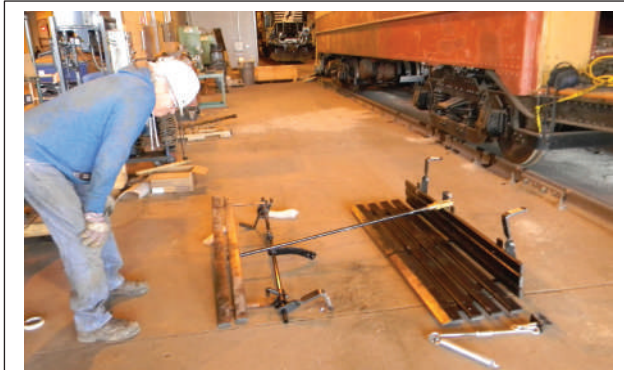
Figure 88: The Life Guard Fender Kit is set out to determine that all the parts are present and fit properly together. Photo: DSCN3326
