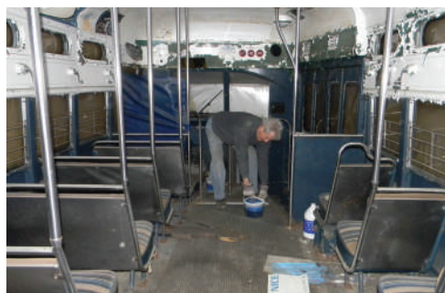
Figure 71: Bob Hooper refreshes the desiccant in PCC # 1 to help reduce moisture inside the shrink-wrapped car. Photo: DSCN3258
