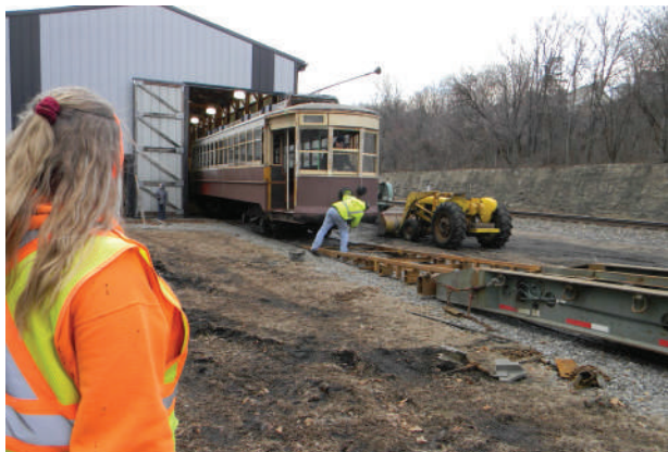
Figure 12: 2651 has just emerged from the car shed under her own power, as Lori Egresi observes. Silk Road driver Don Egresi secures the cable from the flat bed winch which will draw 2651 up the loading ramp onto the trailer. Photo: Tony Hall DSCN3197
