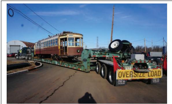
Figure 31: Having entered the property on an easterly heading, our rig has made a right turn passing before the ill-fated Quonsets. Now we are reversing onto an easterly heading preparing to cross the eight lead tracks to the main building. Note the steerable rear bogey, making the required moves possible. Photo: Bob Hooper DSC0449
