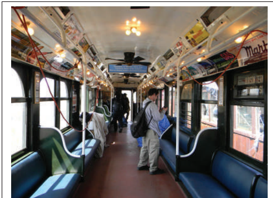
Figure 42: For a few years in the late 1960s, these fine old cars served the World Trade Center, until being displaced by the “K” cars. Note the “compromise roof” which had a limited but significant presence in New Jersey. Photo: DSCN3357
