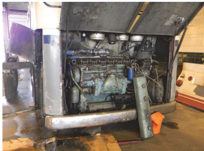
The J411 engine has been rebuilt and is awaiting a new radiator to come.
