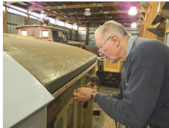
Using his precision claw hammer, Hank Kaminski makes meticulous adjustments to the bonnet plate extensions he has fabricated.
