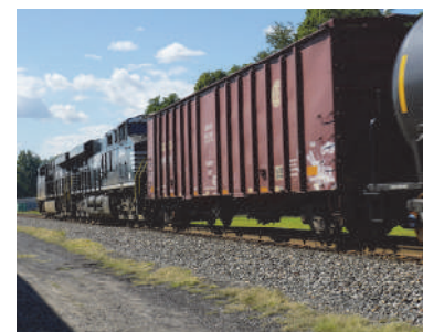
Oil unit trains are so heavy NS adds a distributed power pusher to east bound trains.
