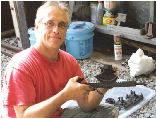
Jim Tomczyk shows off the cleaned rack and pinion gear for the door engines
