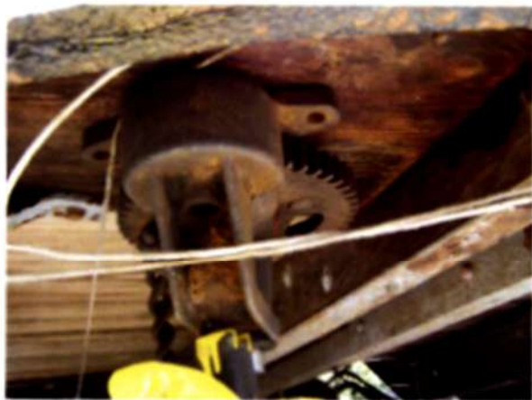
Hand brake chain winder is held in place temporarily with a jack and ropes.
