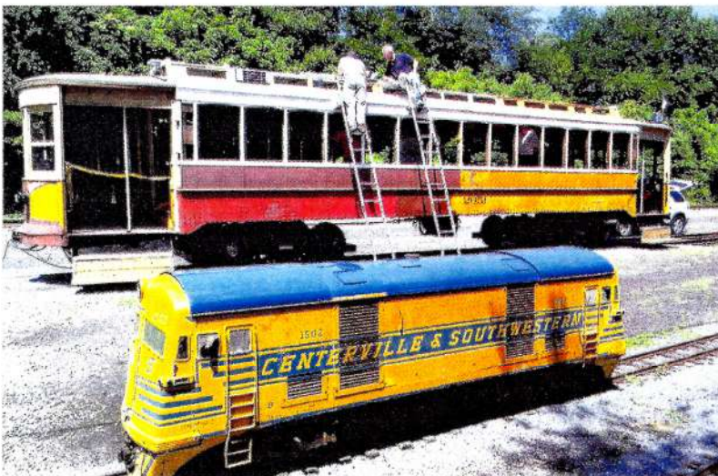
Following Hank Kaminski's expert example, Bob and Jim continue to prepare roof ports for south side ventilators. Double-ended C&S # 1502 basks in the summer sun, enjoying its unaccustomed outdoor exposure. Needed mechanical work will see it back in service next season.
