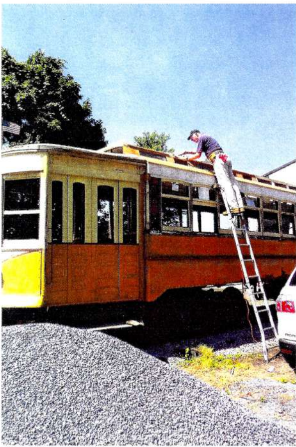
(Upper left) Hank climbs to even greater heights as he tweaks the first ventilator portal to achieve a perfect fit. (Upper right) Bob backs him up from the inside so that the first ventilator is properly fitted.
