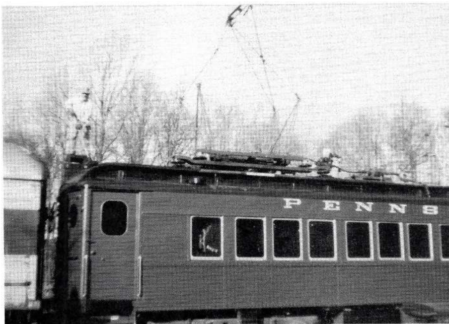
The culmination of a summer's worth of scraping and priming the roof of car 413, saw a coat of high-gloss black enamel applied to the surface. Tony Hall and Bob Landwherle put the finishing touches on some of the last unfinished sections. photo by Frank S. Miklos
