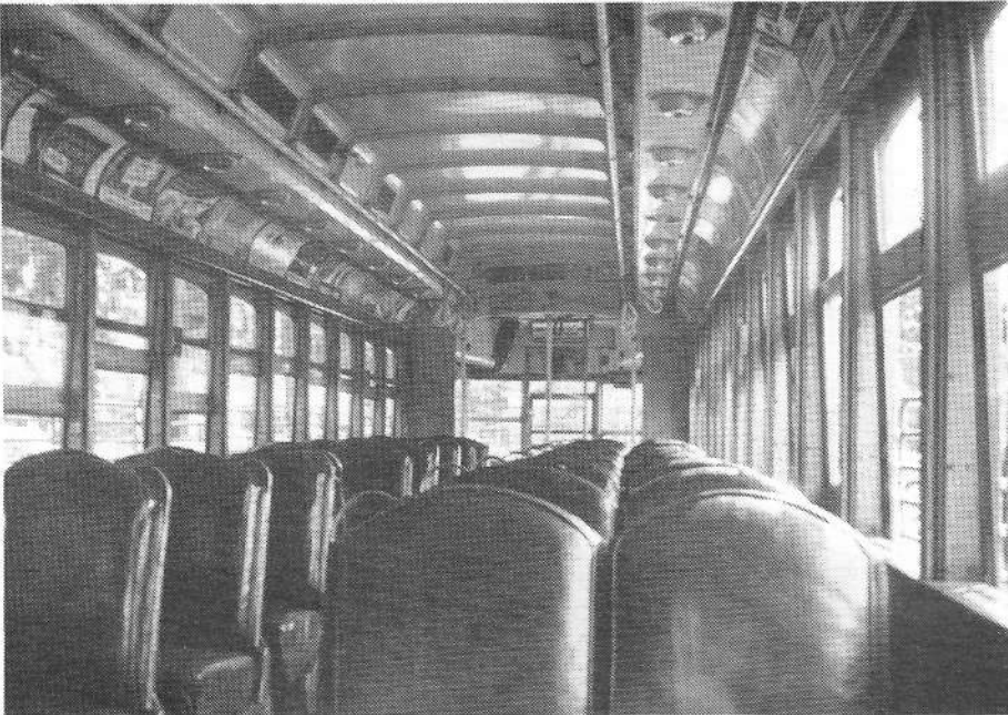
Interior of rebuilt car 2614 in August 1949 shows the leather walk over seating that was retained after the other experimental items were removed. Note the P.C.C. type light fixtures.
