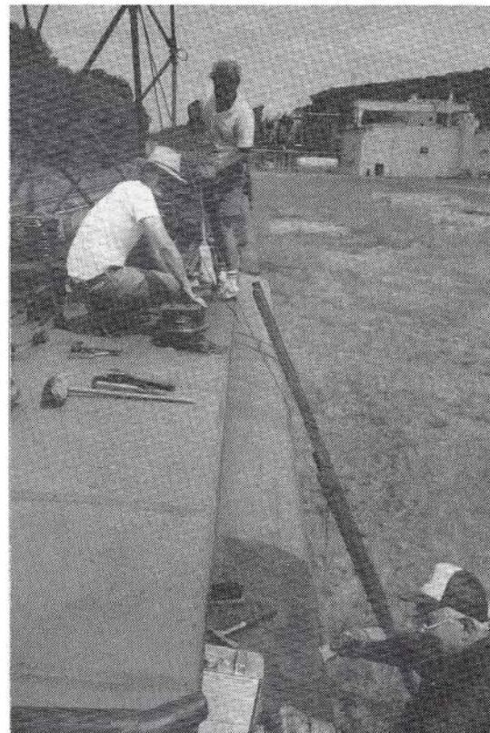
Bob Lanwehrle, Bob Hooper and Frank Miklos prime the roof of PRR MP54 #437.
